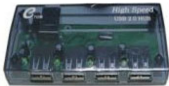
Figure 3: A USB hub can expand a single USB port into many ports.
